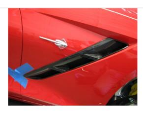
5. Place the new carbon vent to the fender and secure it with 3x8mm nuts, and reinstall the wheel well line screw and splash guard back. Repeat step to other fender.
