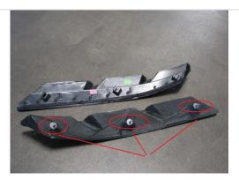
3. Once you have the vent removed off the fender, locate all 3 studs on the vent, and transfer them over the carbon fiber one.
