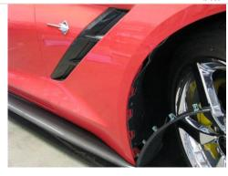
1. Remove the wheel well plastic splash guard off the front fender.
