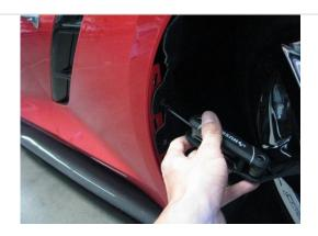
2. Unscrew all 3 torx screws holding the wheel well liner. By opening up the liner, you can reach in with 8mm socket or wrench, remove 3 nuts that holds the fender vent in place.
