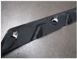
4. Tips: By putting a masking tape to hold the stud in place will help these studs not to slide out of the vent while you try to install it back to the fender.
