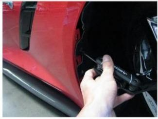
Then you can remove the vent off the fender
