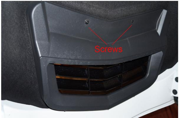
• Remove the hood liner by removing 6 plugs using the plastic plug removing tool (AutoZone has this tool for \$6 or so). You can use small flat head to lift up the plug to slide in your pry tool.
