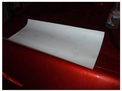
Wet both of your hands and lift up one of the corner and find the stripe cut out corner. Fold it a little bit at the stripe cut out corner to pop out the stripes. Using 1 hand holding down the stripe on the flat wet surface and another hand peeling off backing paper. Make sure your hands are wet so the vinyl will not stick on your hand. Since the vinyl sticks a bit on wet surface, you can use both hand to peel off the backing paper if need to.
