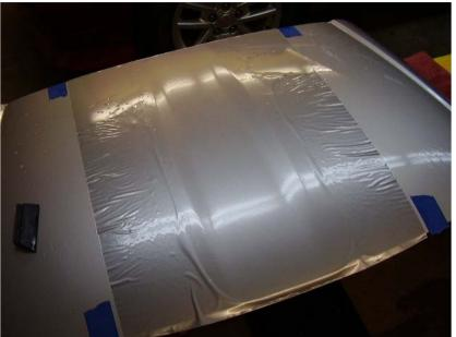
Squeeze the from the middle out side and just always middle to outside for the rest of the stripes. For example, after the 1<sup>st</sup> squeeze at the middle, you will be at the center of the stripes likes this below picture. The next squeeze will be the middle from 1 end to where you just squeezed ©
