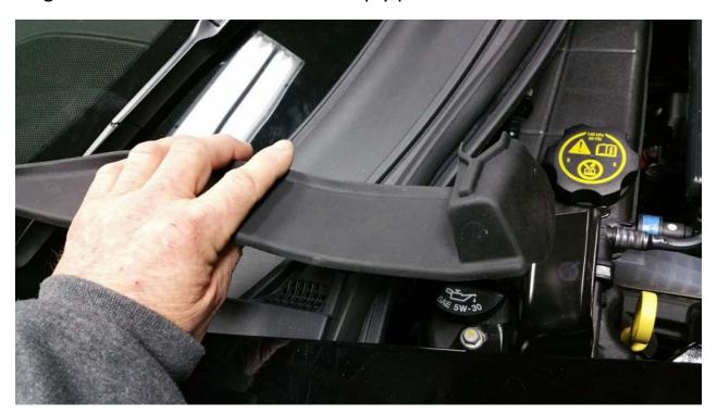
• Pull up on the windshield valance and remove bolt under there.
