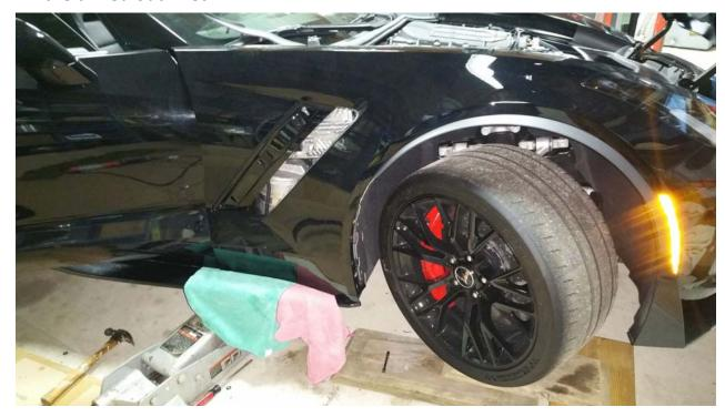
Once I got the fender pulled out I could very easily get to the hardware from the wheel well liner.
