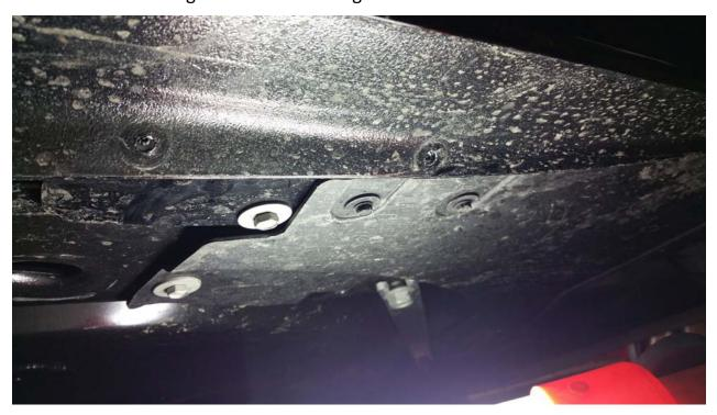
• At this point the rear of the fender is free. You might need to slide a screwdriver in the front lower portion of the fender-to-underside to release the drilled out rivet.
