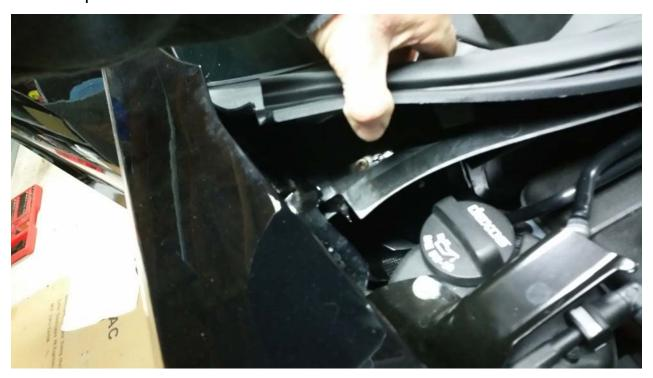
Remove bolt in door jam at top corner of fender.
