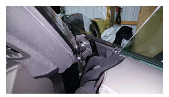
• If you have the side skirts you need to drill out probably 5 rivets and remove one skirt bolt up front because the skirt goes through the fender. You can't pull the back of the fender out if it's still attached to the skirt. I think there are 4 more bolts along the bottom holding the fender.
