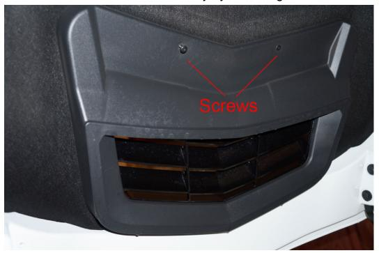
This water drain tray got held by 4 clips so just pull it out.
