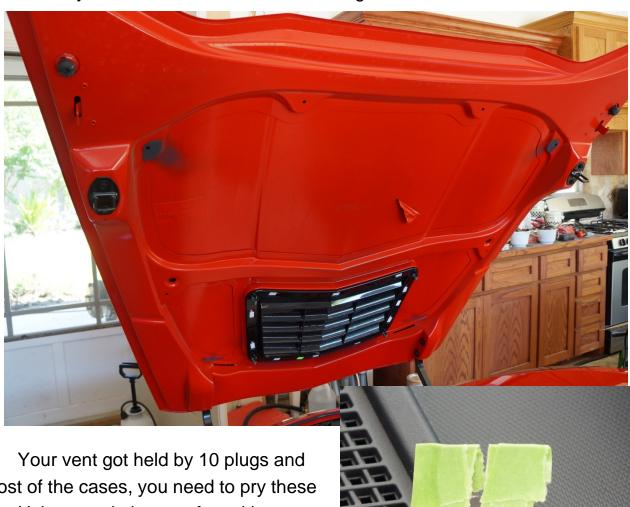
Your vent got held by 10 plugs and most of the cases, you need to pry these out. Using couple layers of masking tape to tape around the head of your above pry tool. These are 10 hard plastic white plugs.
