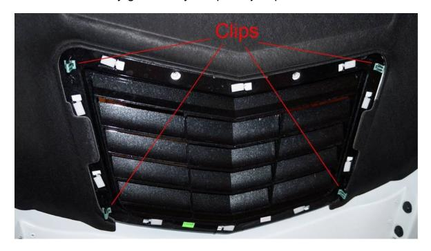
Remove the hood liner by removing 6 plugs using the plastic plug removing tool (Autozone has this tool for \$6 or so). You can use your finger nail or a small flat head screw driver to lift up the plastic plug a bit to slide in the pry tool.
