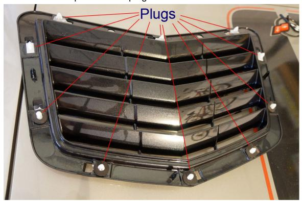
Look around all 4 corners and you would be able to find a corner with more gap to easily slide in your covered pry tool. After slide it in, try your best to pry it as close as possible to the white plug. Don't worry much, C7 vent is super strong so you won't be able to break it! After prying up the first one,
