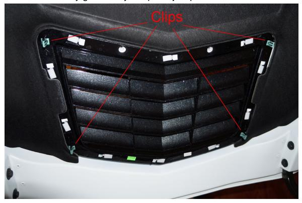
Your vent got held by 10 plugs so also just pull it out after removing the hood liner.
