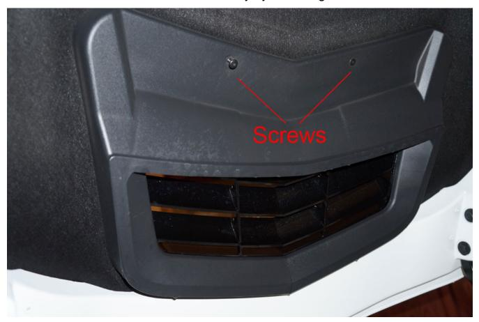
Remove the hood liner by removing 6 plugs using the plastic plug removing tool (autozone has this tool for \$6 or so)
