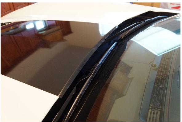
Put back the vent. Remember the hood liner is on top of the vent.
