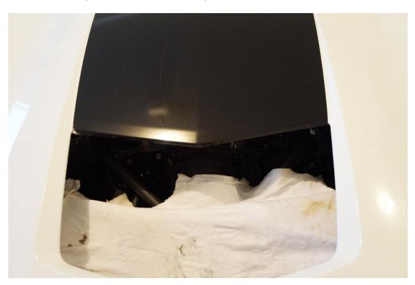
Wait until it dried and bend around the vent hole and top of the hood.
