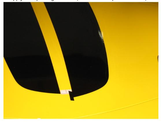
Apply the smaller outer stripes with the spacer still in place
